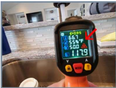
Water temperature at kitchen sink.
